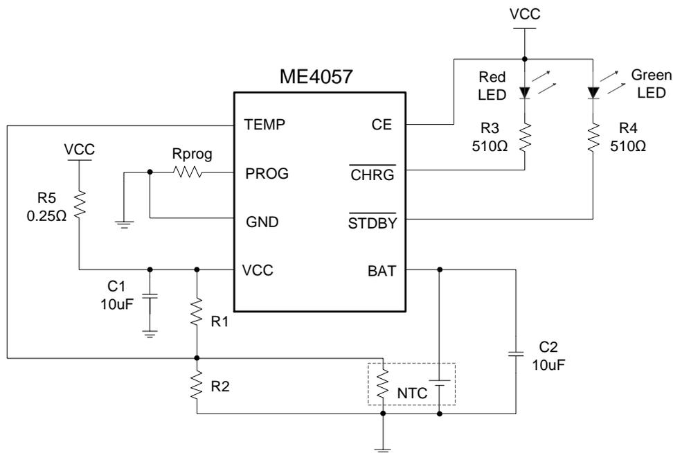
2. Suitable for the application of USB power and the charge of wall adapter
