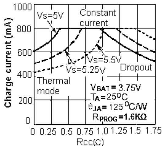
**Fig.4:The relationship curve between charge current with R<sub>CC</sub>**
