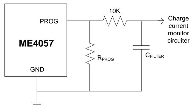
Fig.2 Isolating with capacitive load on PROG Pin
