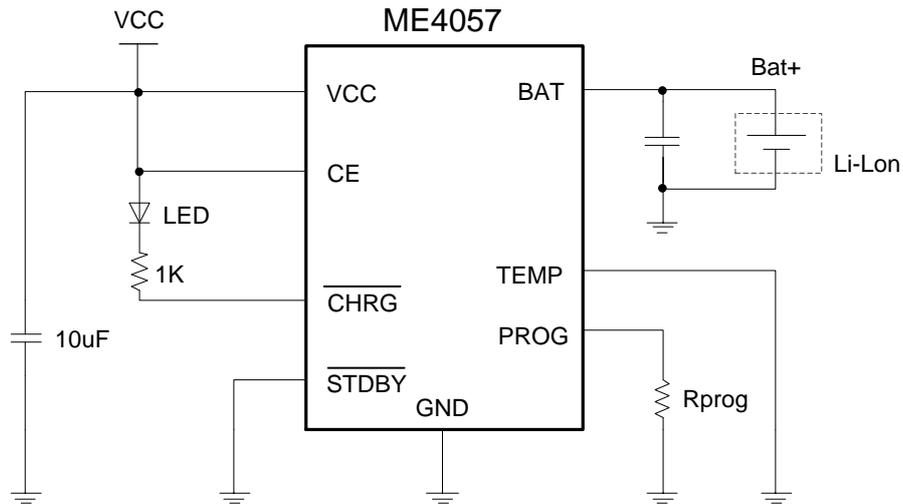
4. Suitable for the application which not need charge status indicator and battery's temperature detection.
