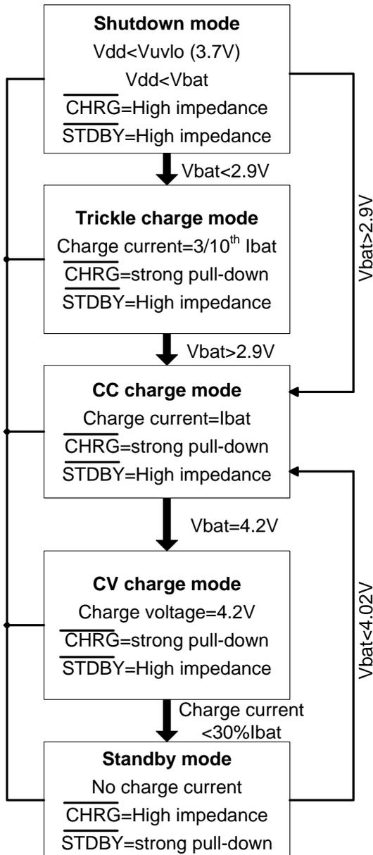
Fig.1 State diagram of a typical charge cycle
